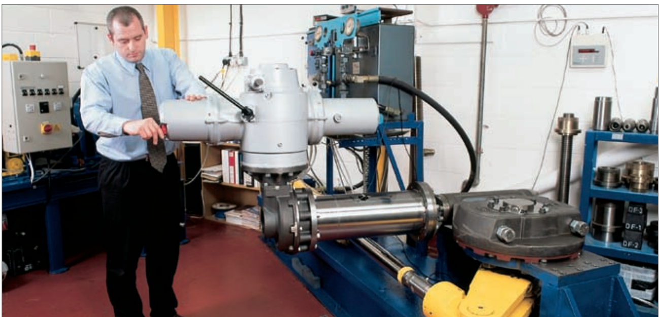
Endurance testing of prototype subsea gearbox
