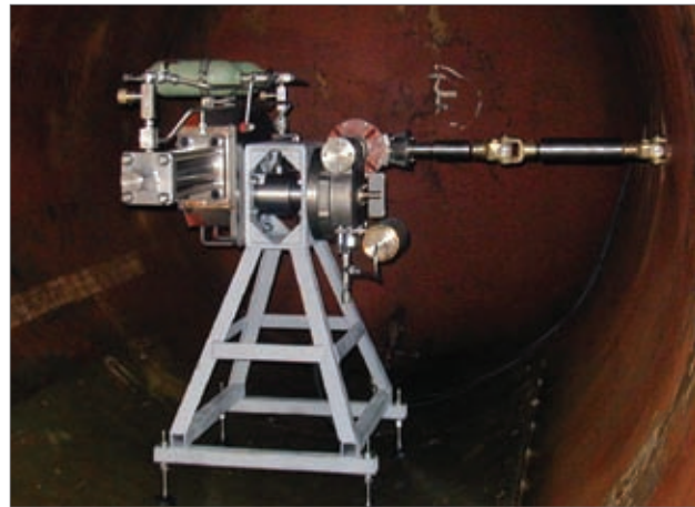
Hydrostatic qualification for subsea gearbox
